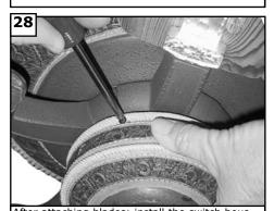
After attaching blades; install the switch housing with the three screws previously removed.
